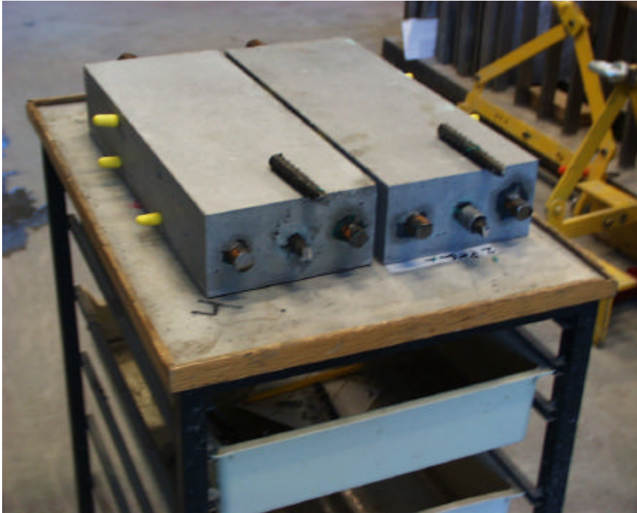
Figure 5 Pull-out specimens with 12 mm bars after testing at 3 days.
